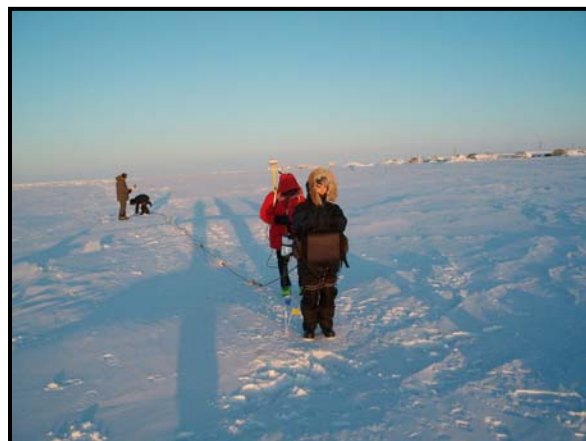
Left to right: Gaven Burnett, Biyuan Zhao, Jason McLarty, and Ashley Taylor use the OhmMapper resistivity array and the GPS backpack unit.
